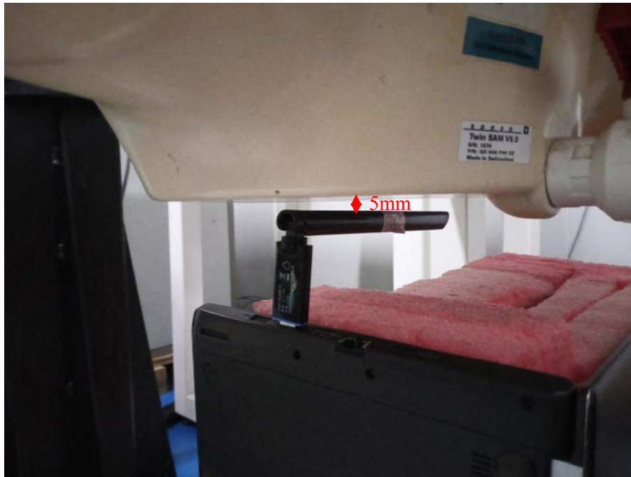
Body Top Setup Photo(5mm)
